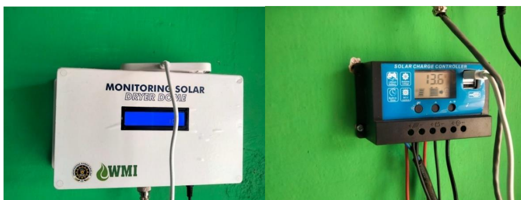
Gambar 3. Sistem monitor suhu dan kelembaban serta solar charge controller
